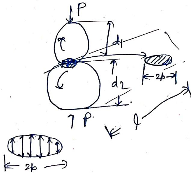
$$b = \sqrt{\frac{2P(1-\mu^2)}{\pi l} \left( \frac{1}{E_1} + \frac{1}{E_2} \right)} \quad \text{--- (b)}$$
