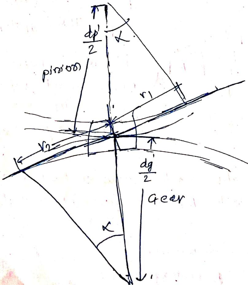
figure shows the contact between two meshing teeth at pitch point. The radii  $r_1$  &  $r_2$  are replaced by radii of curvature at pitch point.
