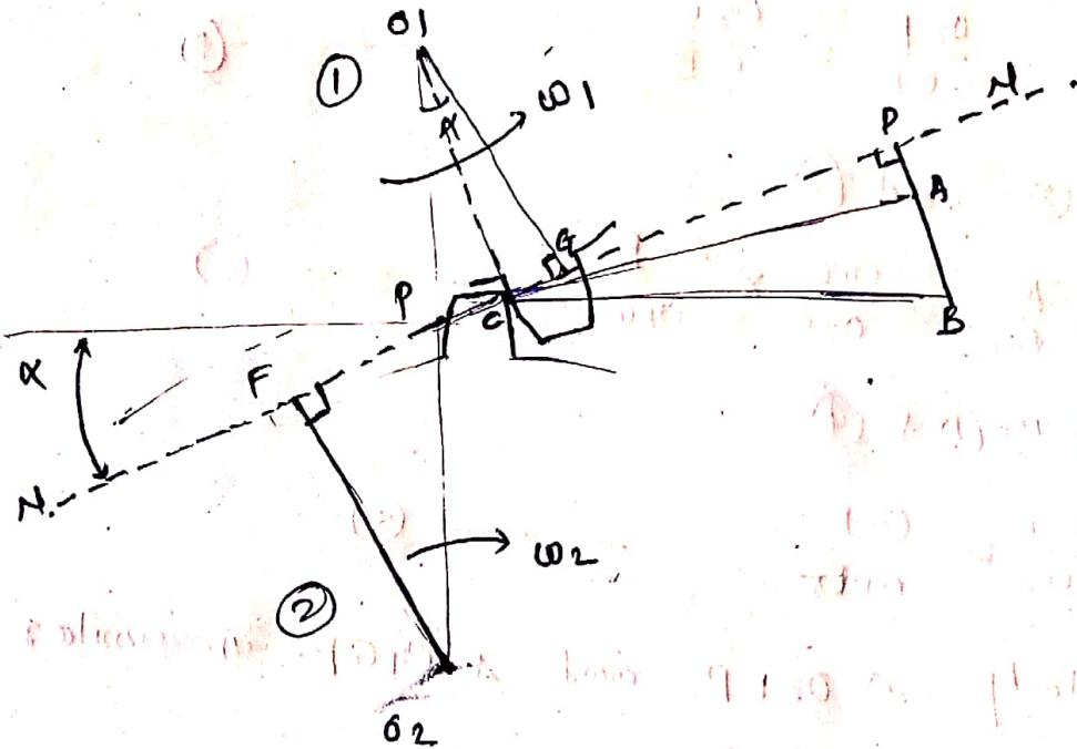
$O_1, O_2$  = centres of two gears which are rotating with angular velocities  $\omega_1$  &  $\omega_2$  resp.
